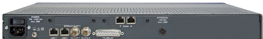
MAGIC THipPro Pure rear view with optional Dante® module and redundant power supply upgrade
